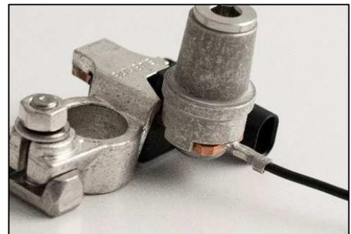
Now mount the vessels ground cable (the one that has been attached directly to the battery before) onto the battery pole adapter on the IBS.
