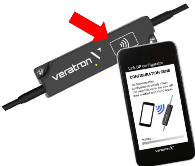
1. Launch the "Link Up Configurator" app and read the current configuration of the LinkUp device by "tapping" the smartphone onto the LinkUp wireless area (indicated by the red arrow).
