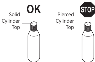
FIGURE 3 CO 2 CYLINDER CHECK
