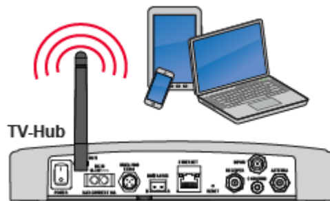
Figure 3-3 TV-Hub Wi-Fi Connection (TV-Hub A+ shown)
