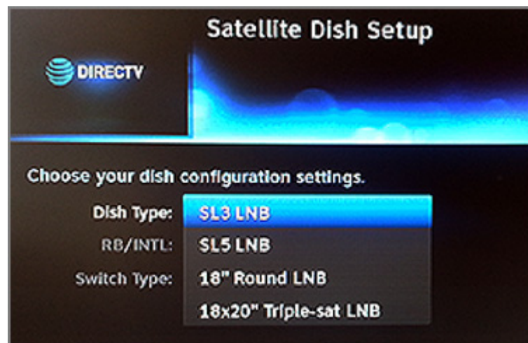
Figure 5-7 Dish Type Menu on DIRECTV Receiver (Example)
