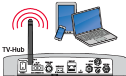
Figure 2-5 Wireless Connection to TV-Hub Web Interface
