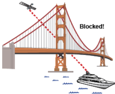
Figure 2-2 Example of Satellite Blockage
