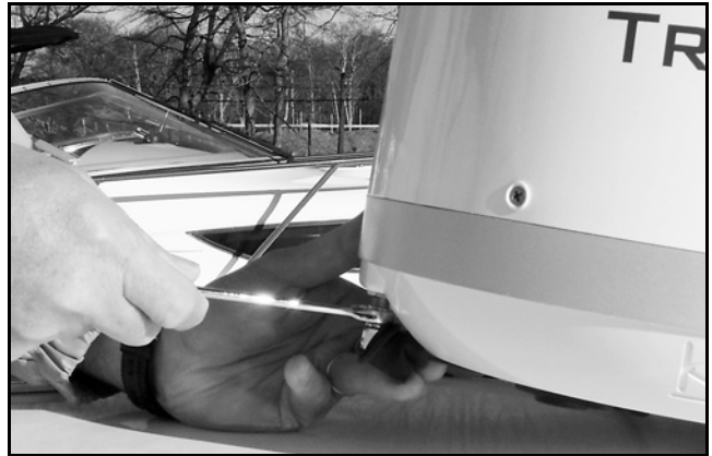
Figure 11: Connecting the Antenna Cable
