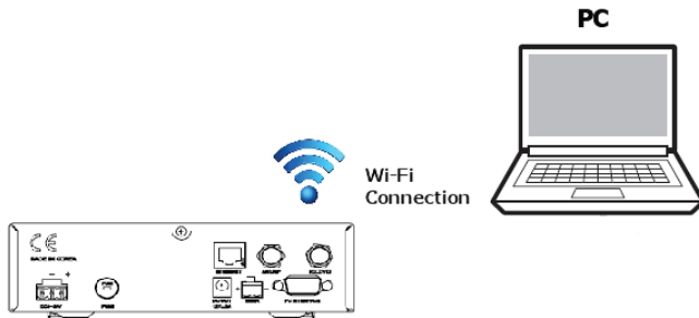
Figure 27 : ACU to PC Wifi Connection
