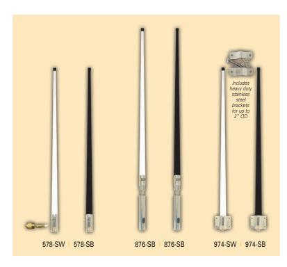
In conjunction with the USCG Automatic Identification System (AIS) requirements for commercial vessels, Digital Antenna created a series of 4' AIS antennas that meet the exacting AIS frequency requirements. Designed with a low 1.5:1.0 SWR ratio from 159-162 MHz, Digital Antenna's 4.5 dB gain AIS antennas offer unsurpassed durability and performance compatible with all AIS transponders.
